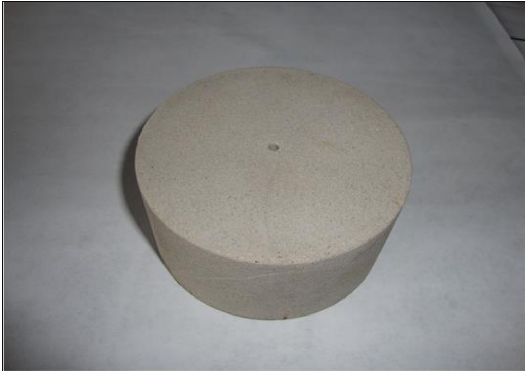
Figure 3-2, a 4-inch sandstone cores sample post CO 2 sweep with 20% oil and remainder CO 2 and water
