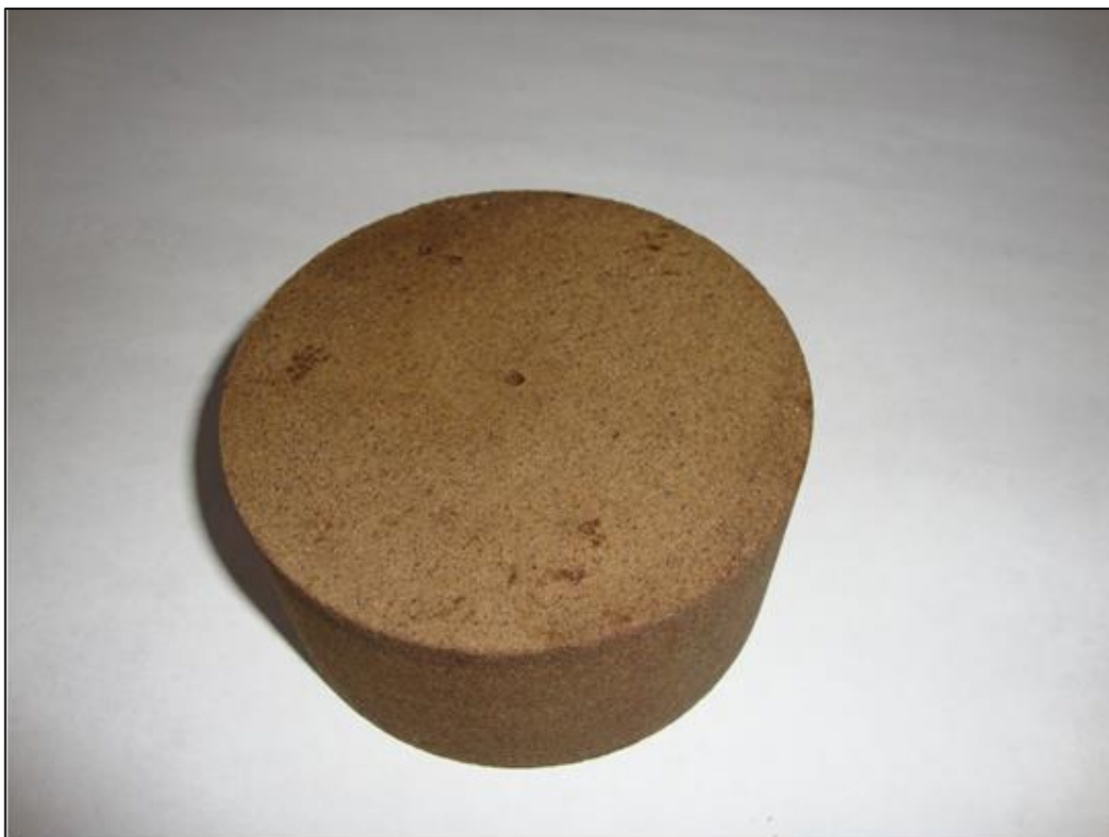
Figure3-1 a 4-inch sandstone core sample with 35% oil saturation and water
