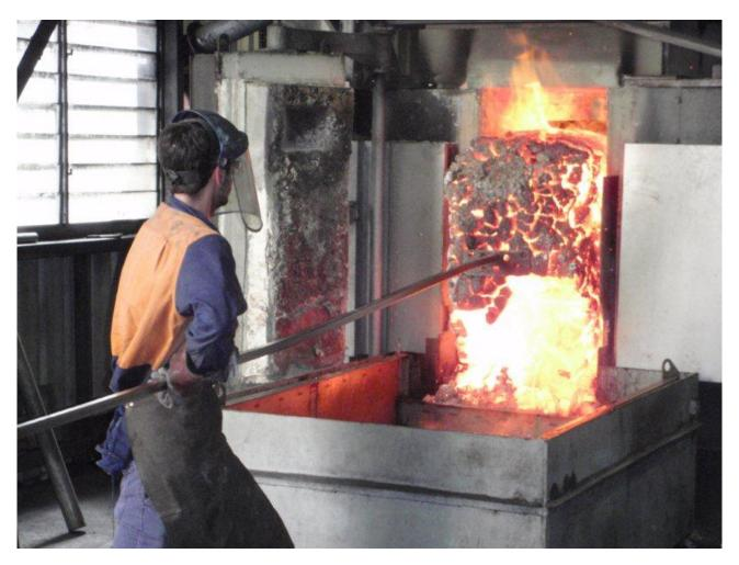
Coke oven testing of New Lenton Coal
