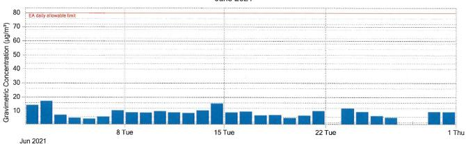
Figure 1: Jondaryan Township TSP continuous monitoring 24 Hr average results for June 2021
