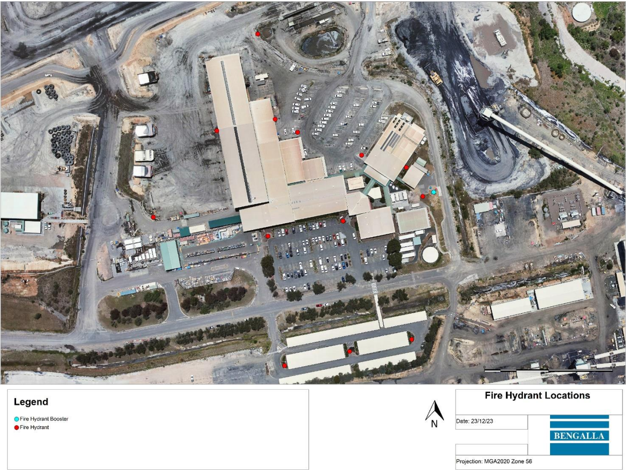
FIGURE 6: Fire Hydrant and Extinguisher Locations
