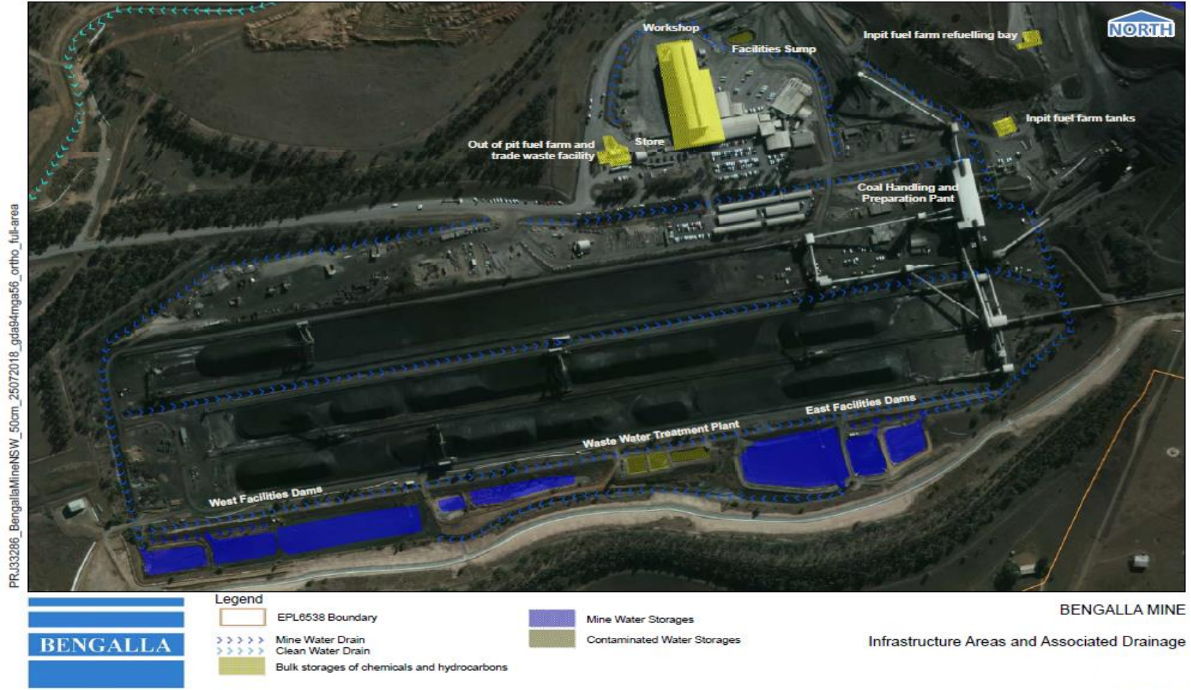
FIGURE 4: Infrastructure Areas Drainage and Storage
