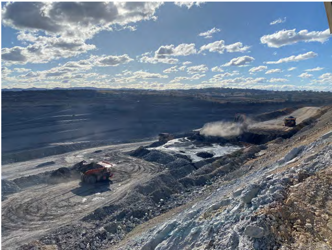
Plate 26 - Waste Rock Dumping on Reject Cells
