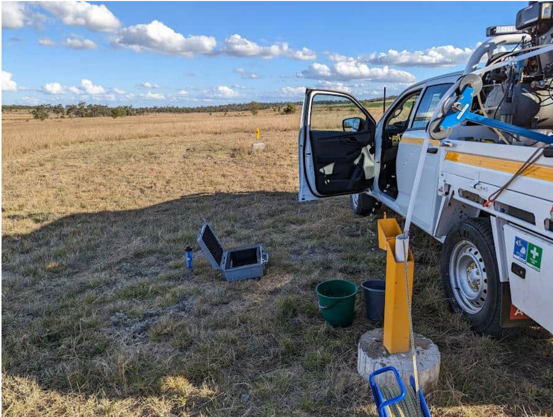
Photograph 03: GW22A and GW22B sampled on 11/05/2023 with Bennett Pump
