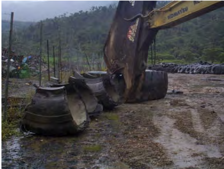
Figure 6.2.1 Hydraulic shears sectioning tyres (photo Gary Moffat)
