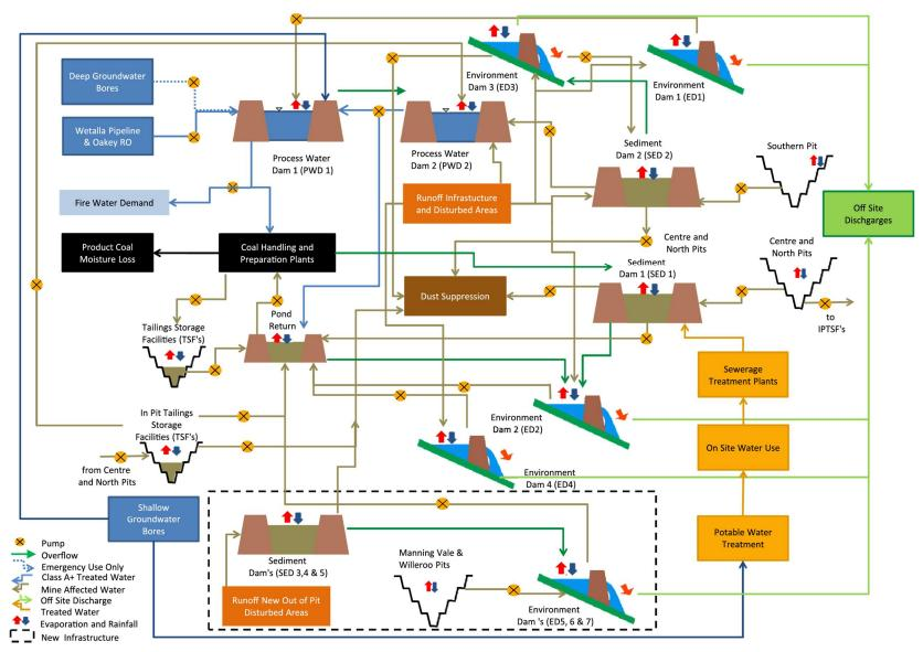
Figure 3–27 Water Management System Schematic
