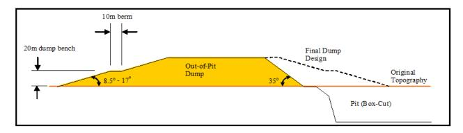
Figure 3–17 Spoil Dump Conceptual Design Plan
