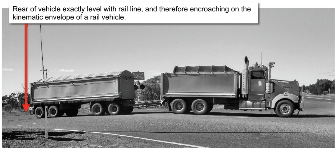
Figure 7: Two-trailer vehicle observed during site visit overhanging level crossing whilst waiting to turn right onto Warrego Highway
